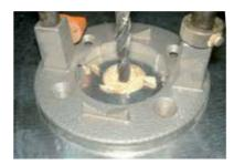
• Drill the metal sheet with a sufficient diameter (for example 30mm), then pre-drill a hole for the hanger bolt with 0.7 x diameter (for M10: 7mm, for M12: 8.5mm). Use a corresponding drill template to maintain the vertical alignment.
