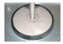
Placing of the sealing disc
