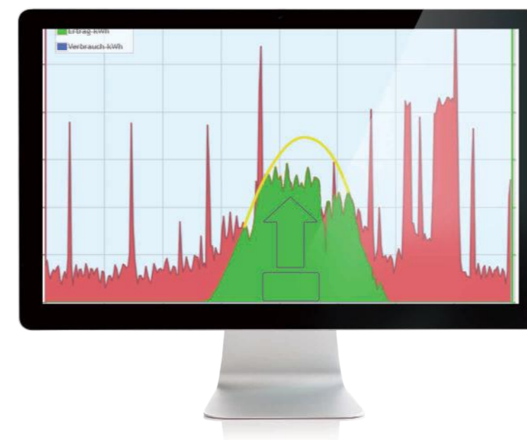
The utilization of solar energy is increased when controllable appliances are activated.
