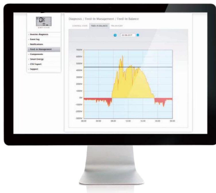
Feed-in Management - feed balance: The times when there was a grid feed and when electricity was purchased from the grid can be seen at a glance in this graph. Negative (red) values indicate that electricity was purchased from the grid and positive (yellow) values that there was grid feed.
