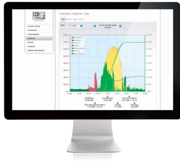
Daily overview: The battery system is charged when there is a surplus of PV power at the plant (light green) and is used when there is not enough PV power to cover consumption needs, preventing the need to purchase electricity from the grid.
