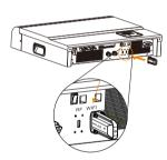
\*Notes: Inserting Pocket Wifi 2.0 into "RF" port or "Upgrade" port may lead to system failure.
