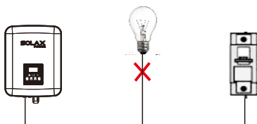
Incorrect Connection between Load and Inverter
