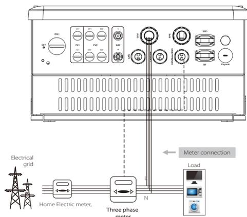
Communication interface between inverter and meter is RS485 with a RJ45 connector.
