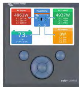
Color Control panel, showing a PV application
