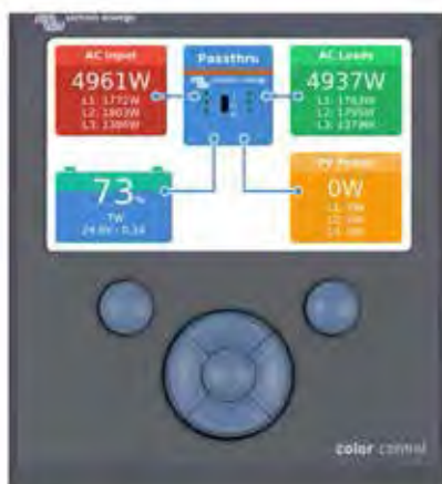
Color Control panel, showing a PV application
